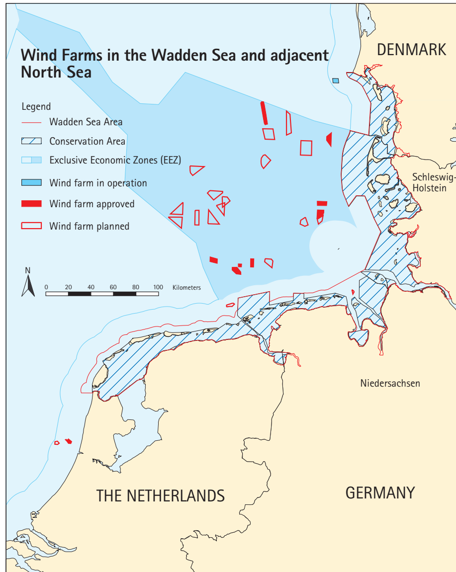
Figure 2.9.1: Offshore wind farms in the North Sea adjacent to the Wadden Sea (status February 2005). In the German EEZ, only pilot projects are shown, further extension areas of wind farms are not indicated.
