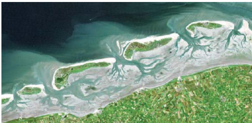
Figure 4: Typical saw-tooth bar system in front of a barrier island of the East Frisian Wadden Sea.
